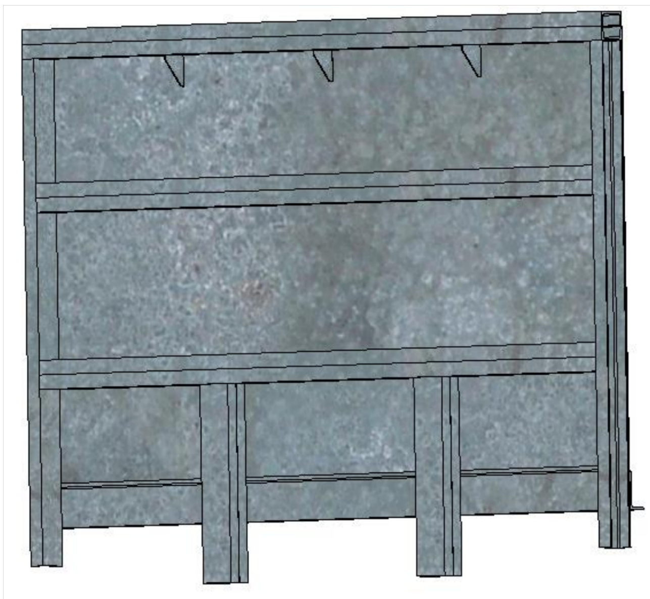
Figure 3.1. End wall of freight wagon model 12-4745. Existing design scheme
