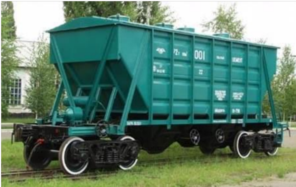
Figure 1.44 - General view of the wagon hopper model 19-758 for the transportation of cement
