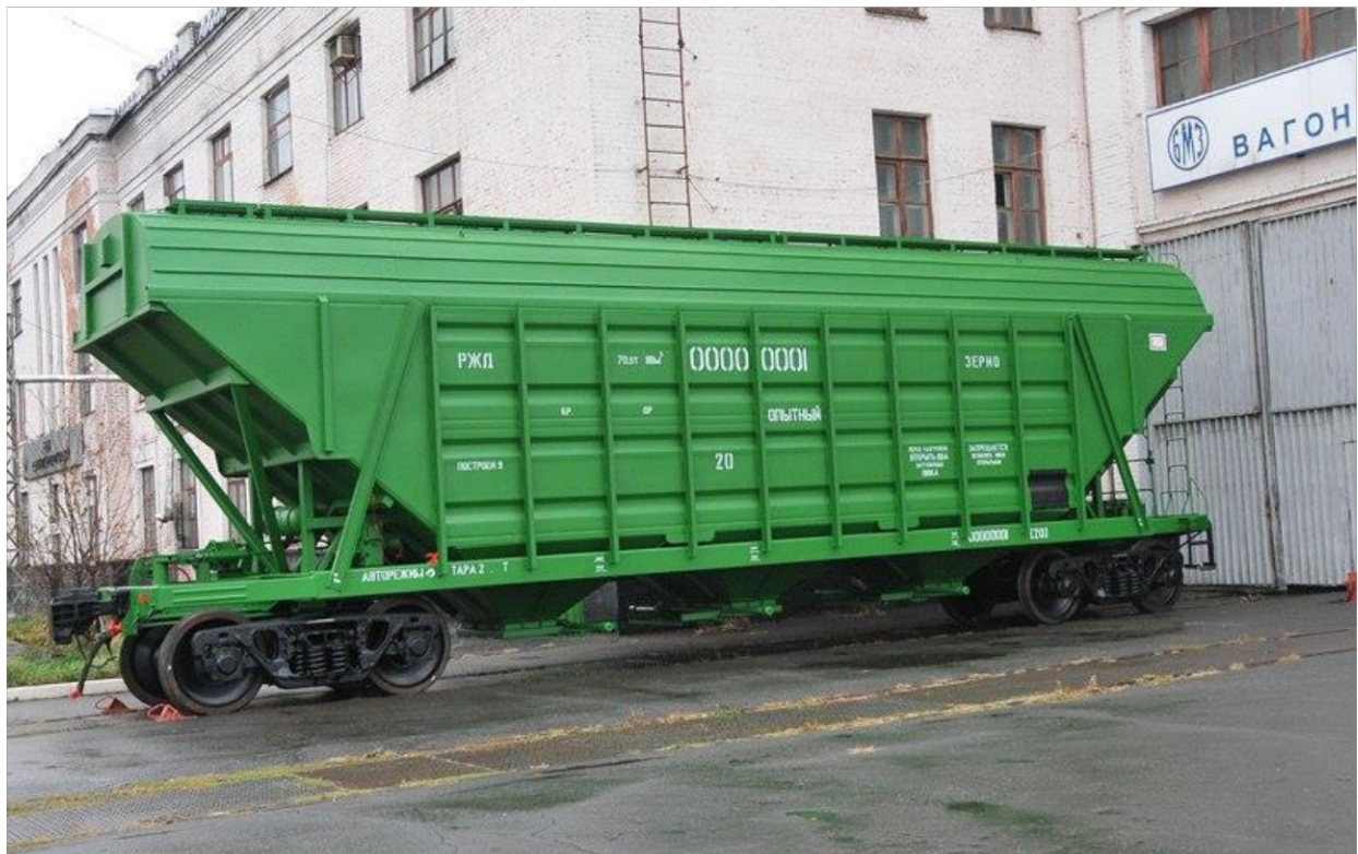
Figure 1.39 – General view of the 19-3058 model hopper wagon for transporting grain
