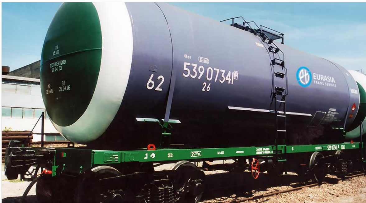
Figure 1.79 – Tank wagon model 15-1443-06 for transportation of light petroleum products
