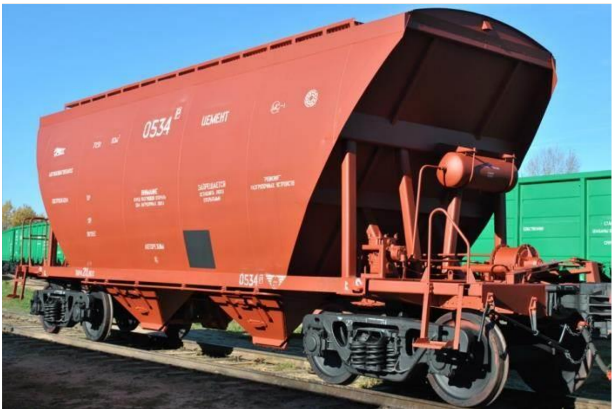
Figure 1.51 – General view of the 19-9862 model hopper wagon for transporting cement
