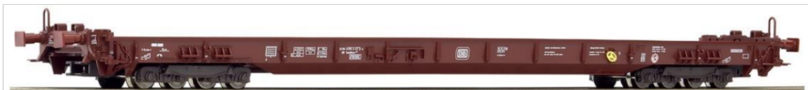
Figure 1.75 – A flat wagon with a lowered loading platform for the transportation of road trains according to the "RoLa" system
