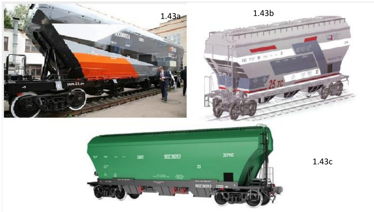
Figure 1.43. - Hopper wagons of the new generation: a - hopper wagon for goods that require protection from atmospheric precipitation; b - hopper wagon model 19-9549-01 with increased body volume; c - hopper wagon for grain transportation model 19-6870
