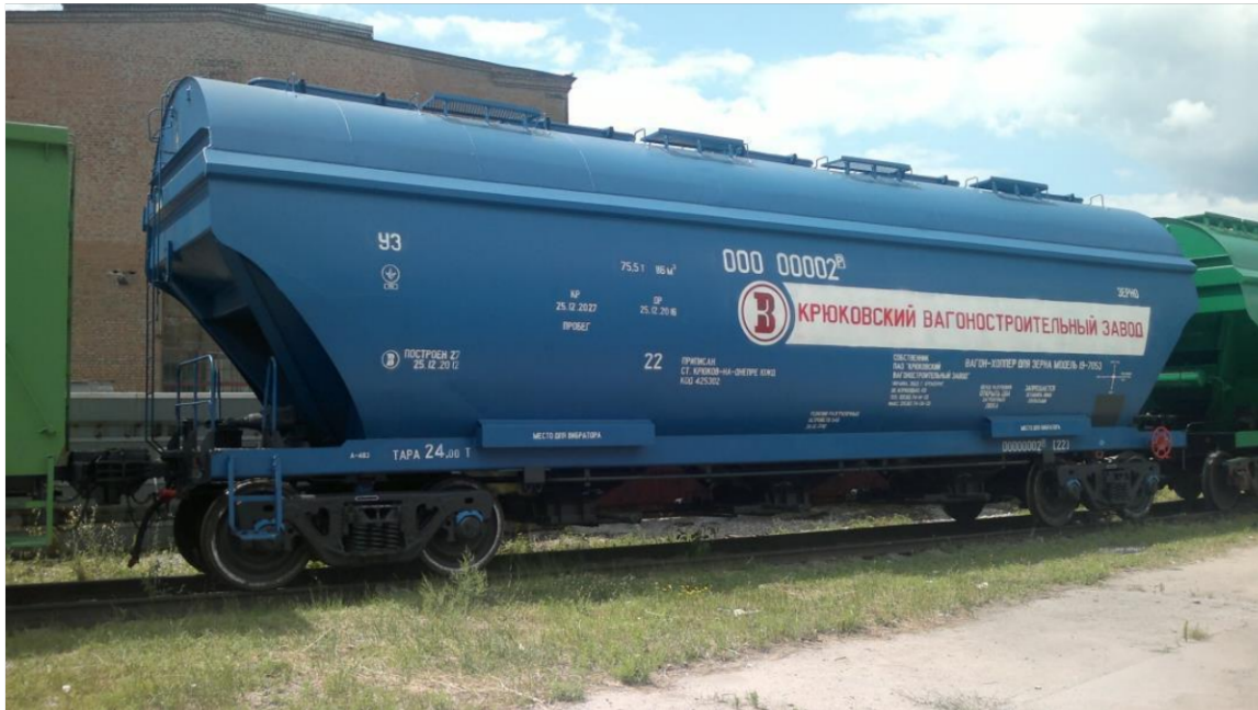
Figure 1.33 - General view of the hopper wagon model 19-7053 for transporting grain
