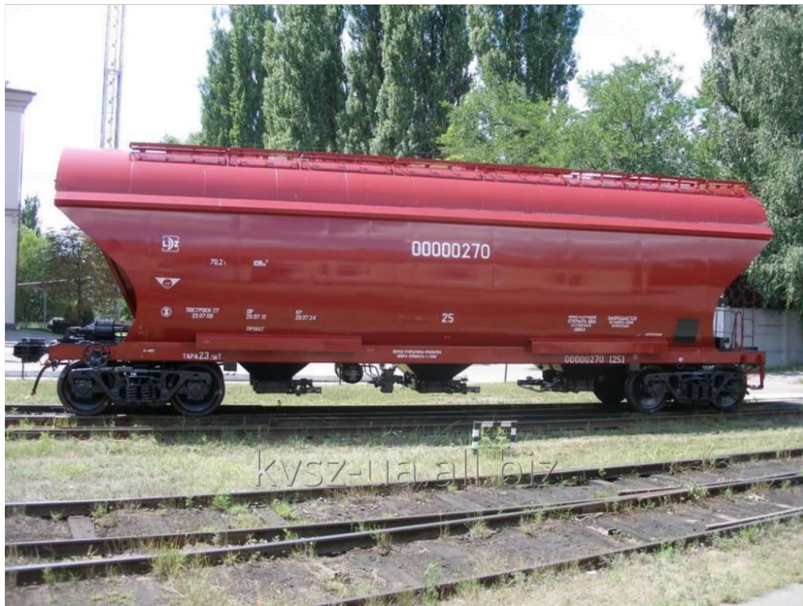
Figure 1.29 – General view of model 19-7016 wagon for the transportation of bulk goods
