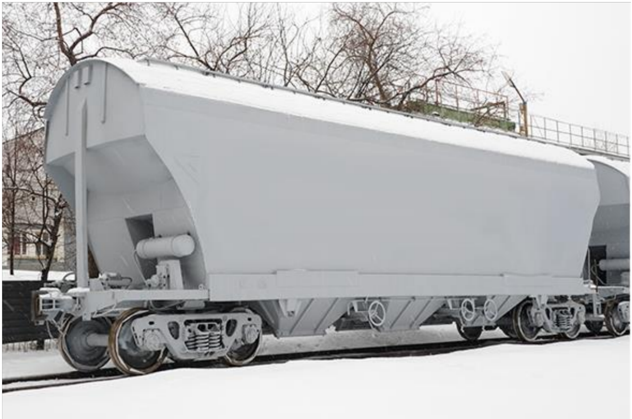
Figure 1.36 – General view of the 19-6870 model hopper wagon for transporting grain
